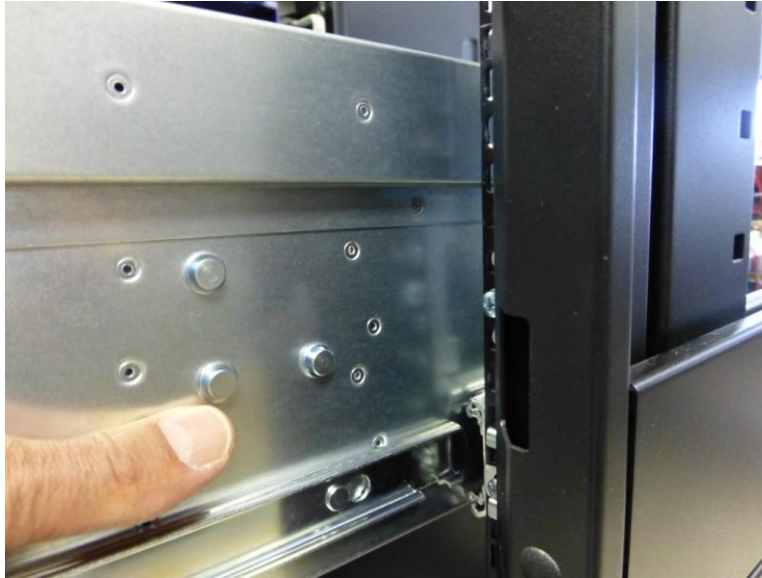
Figure 14. Sliding IceBreaker 4960J Chassis Rail into Middle Rack-Mounted Rail
