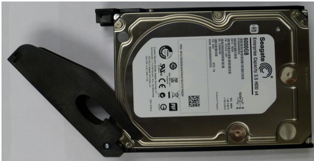
Figure 26. Disk Drive Installed in Carrier
