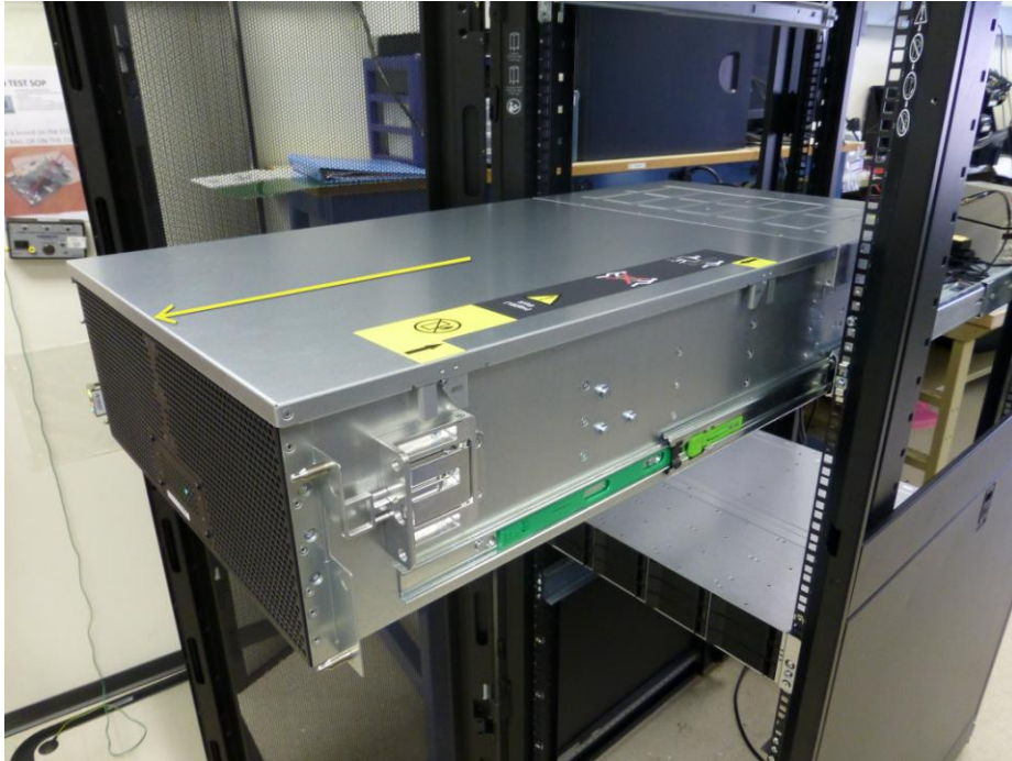
Figure 22. Sliding IceBreaker 4960J Unit Out of Rack
